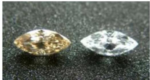
**The colourless stone on the right has been HPHT treated**
