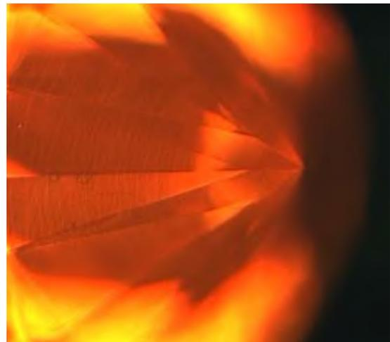
**DiamondView™ image of a CVD synthetic diamond that has not been heat treated after growth**
