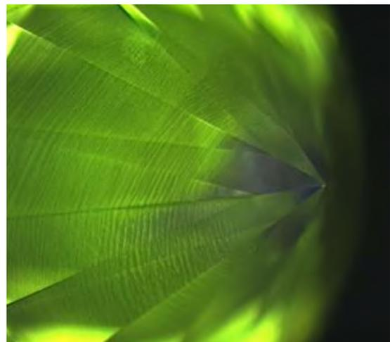
**DiamondView™ image of a CVD synthetic diamond that has been heat treated after growth**
